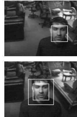
Figure 3: Detecting a person glancing at an article and stepping closer to see more. By gazing at the camera for a longer duration, a person allows the system to capture his face.
