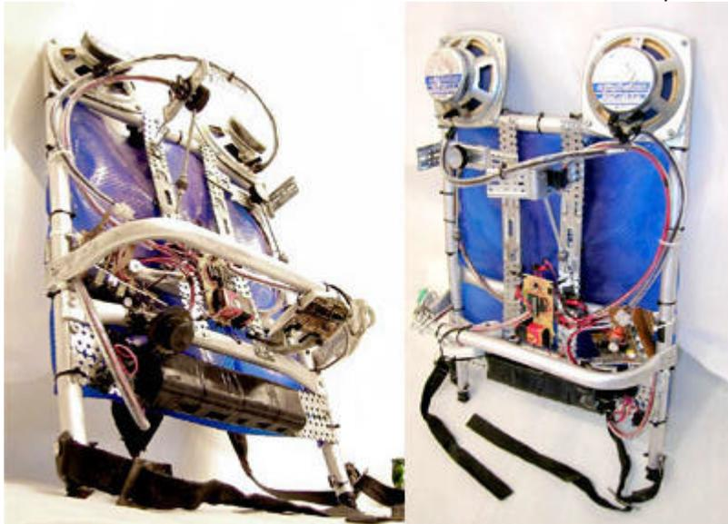
The design of it is quite simple, with breaking off the amplifier from an old radio, and using a cheap microcontroller (Basic Stamp).
